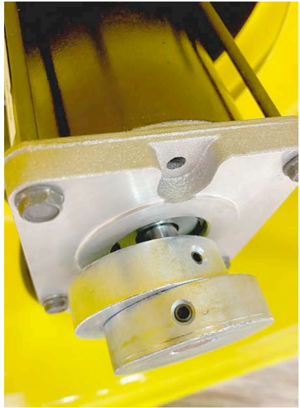
Amplitude adjustment can be made by loosening the bottom weight and rotating as described on the left.
